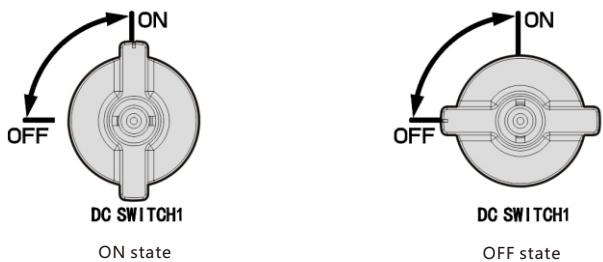
Fig 9.8 DC switch status
